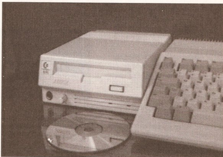
The A570 CD-ROM drive in all its glory. The prototype model we looked at was still badged as an A690. As can be seen, the styling is similar to the A590 hard drive – too bad you can't have both next to each other
